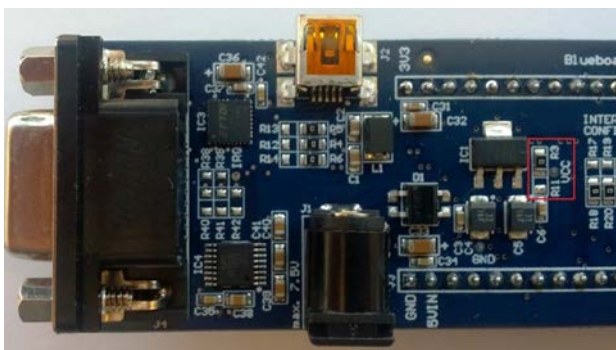
Fig 12. Solder jumper for VCC power supply configuration
